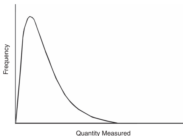
Figure 9020:1. Frequency curve (positively skewed distribution).
